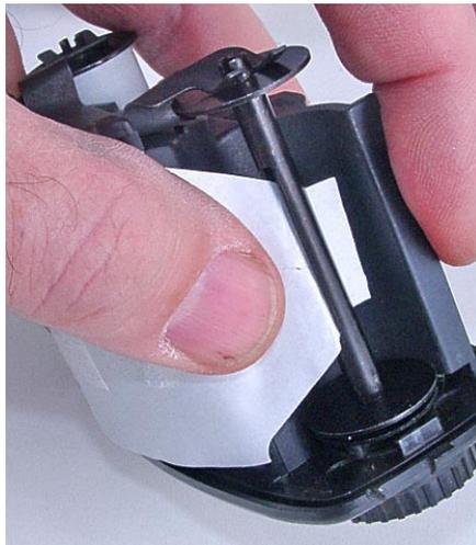
Insert the tongue into the take-up spool slot. Continue to maintain light pressure on the roll of film so it does not spontaneously uncoil. Turn the film advance knob so it grips the backing paper, and begin advancing the film into the take-up chamber.
