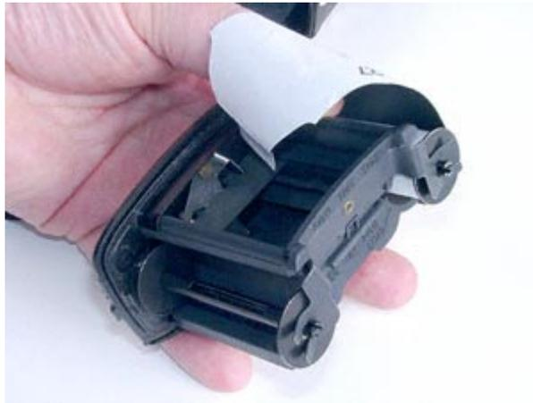
Insert the roll of film into the supply chamber. Press it with a finger or thumb so it does not spontaneously uncoil. Pull out about 10cm (4 inches) of the backing paper and draw it across the film plane.
