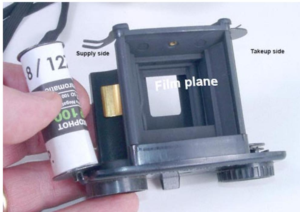
Your camera will have a supply chamber, which holds the unexposed film. It will have a take-up chamber, where you advance the film as you expose it. They will be on opposite sides of the film plane.
