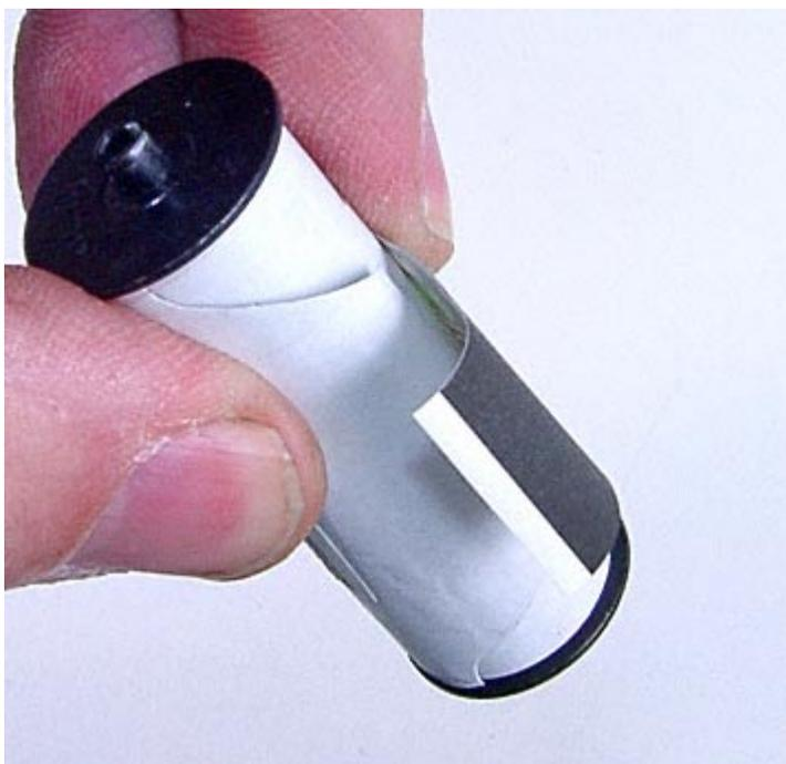
When you have exposed the last frame, wind the film all the way forward. Remove it from the camera and use the supplied gummed seal to seal it shut. Leave the empty spool in the camera for use as your next takeup spool.
