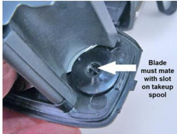
Note that the slot in the end of the empty film spool must mate with the blade on the film advance shaft.
