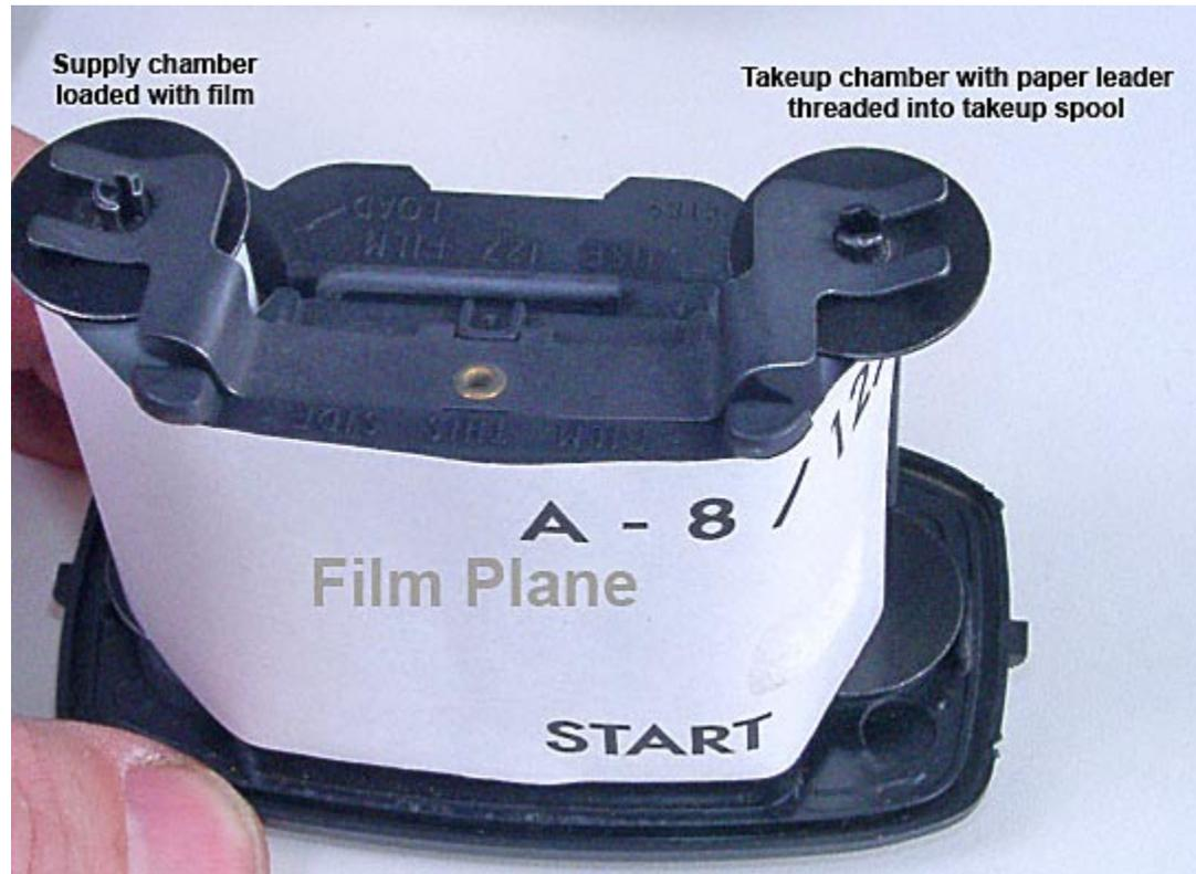
This illustrates how the film feeds from the supply chamber (on the left in this camera), across the film plane, and onto the take-up spool. The word "start" tells you that you are at the beginning of the roll.
